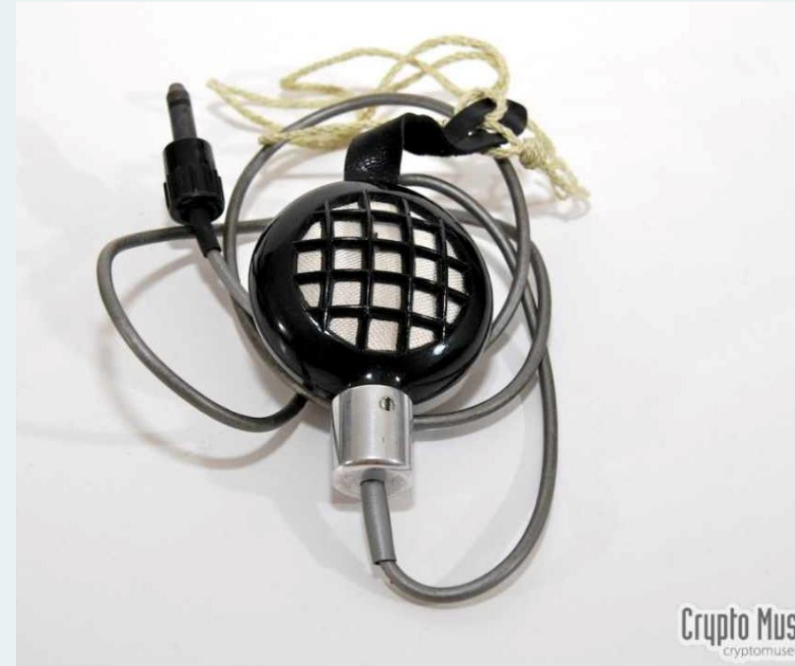
The 'standard' microphone supplied with the Mi-51. Attaches to clothing with a leather strap.
